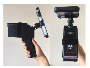
A lightweight and ergonomic assembly combines the two CT007-M and smartphone for comfortable one-handed operation. The Smartphone provides a large display with access to a feature-rich menu. The phone's audio can be played through earphones for use in noisy environments.
