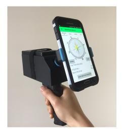
When two CT007-M are connected to the GammaGuard app, the app can compute the direction of the radiation source by comparing the radiation levels detected by the two detectors. The result is plotted on a compass display on the phone.
