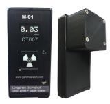
The CT007-M is intended for finding concealed sources of radiation. It features almost twice the sensitivity of standard microR meters at about 15% the size (33,000 CPM/uSv/h). The CT007-M can be used by Border Services personnel to locate radioactive sources in vehicles after portal monitors have alarmed, or they can be used to replace portal monitors. It can be used by law enforcement for detecting and finding concealed radioactive materials.
