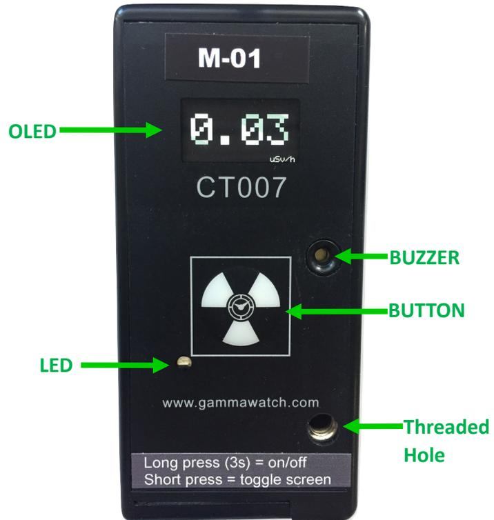
Figure 2.1 CT007-M Front Face Plate
