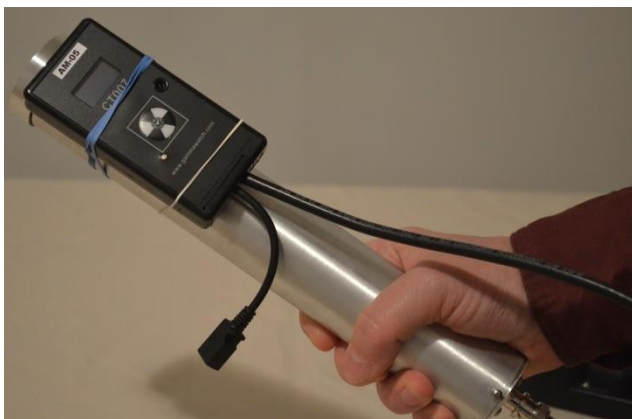
Photo 4: Environmental Instruments AM003 Interface with NaI(Tl) Detector
