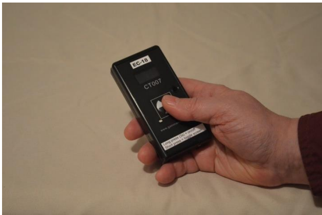
Photo 2: Environmental Instruments CT007-EC Gamma Survey Meter
